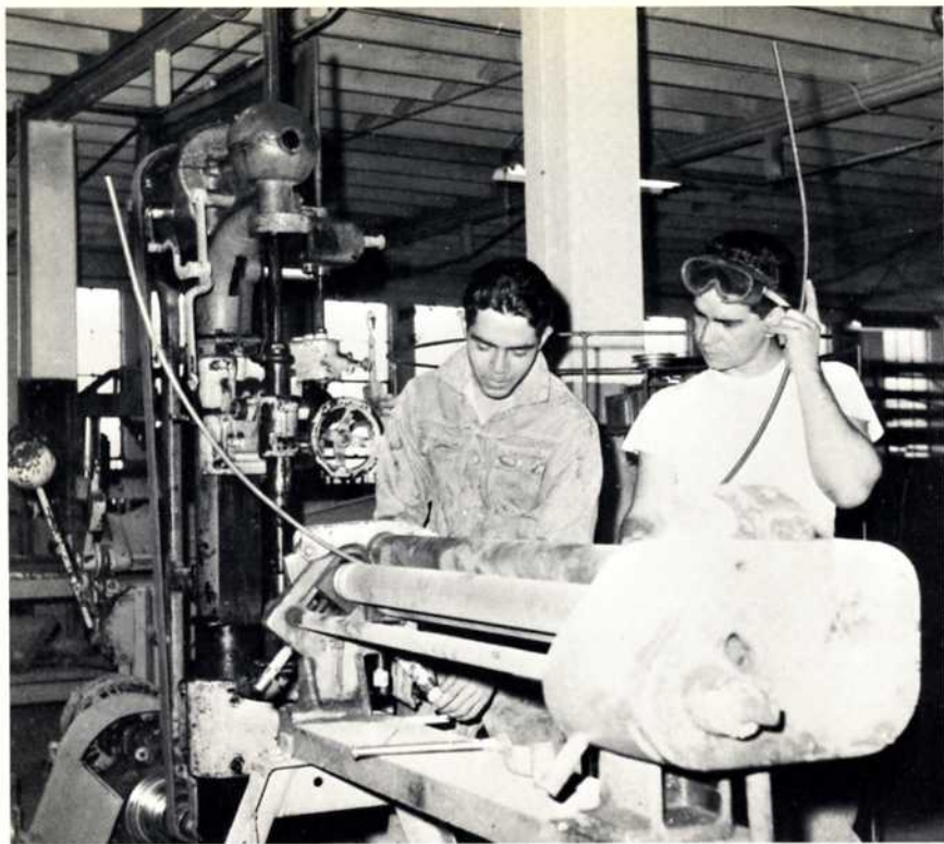
Alfonso Escobedo and Juan Lozano are rolling metal in order to finish their project.
