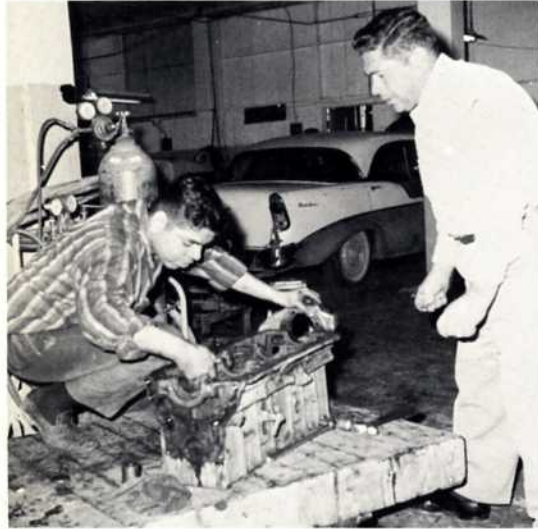
Mr. Cortez explains to Jose Coronado how to remove the camshaft on 6 cylinder engine to install camshaft bushings.
