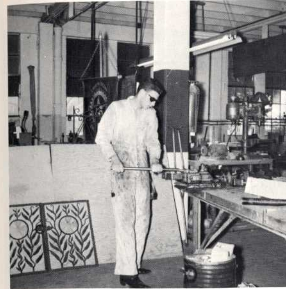
Pete Cabrera is operating a bench bending machine.
