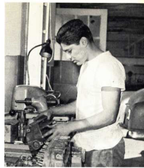
Examining the tappet shaft for defects is Oscar Castillo.
