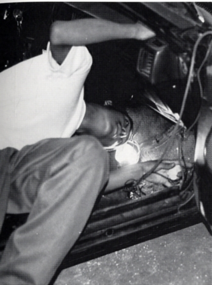
Ramon Madrigal installs an ECM computer.
